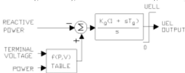
**Fig. 2. Simplified UEL Block Diagram**
