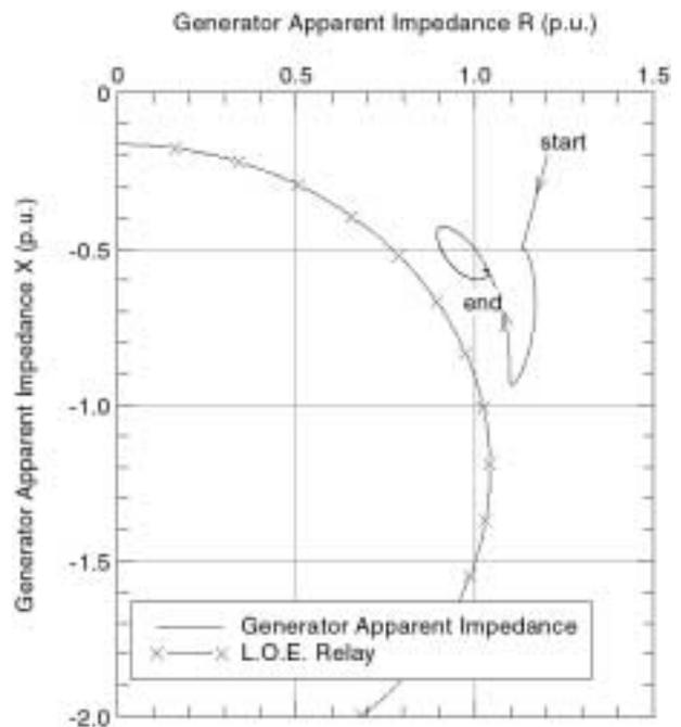
**Fig. 4 LOE Characteristic and Impedance Trajectory**
