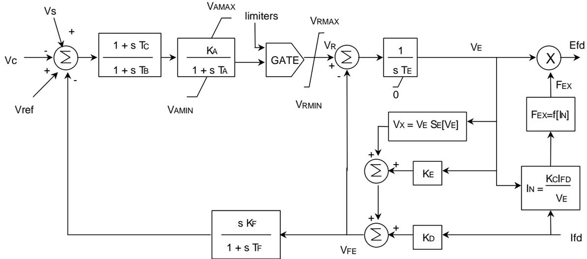
**Figure 3: Excitation System Model Type AC1A**
