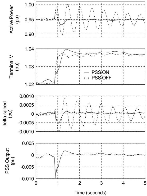
**Figure 9. Power System Stabilizer Test**
