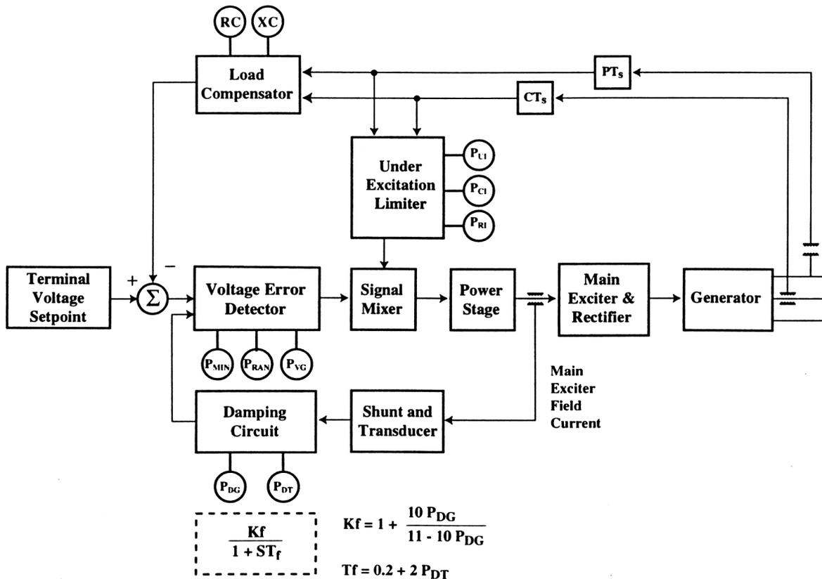
Figure 2: Overview of Block Diagram of Exciter Including External Settings
