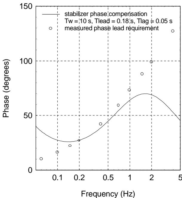
**Figure 8. Stabilizer Phase Lead Requirement**
