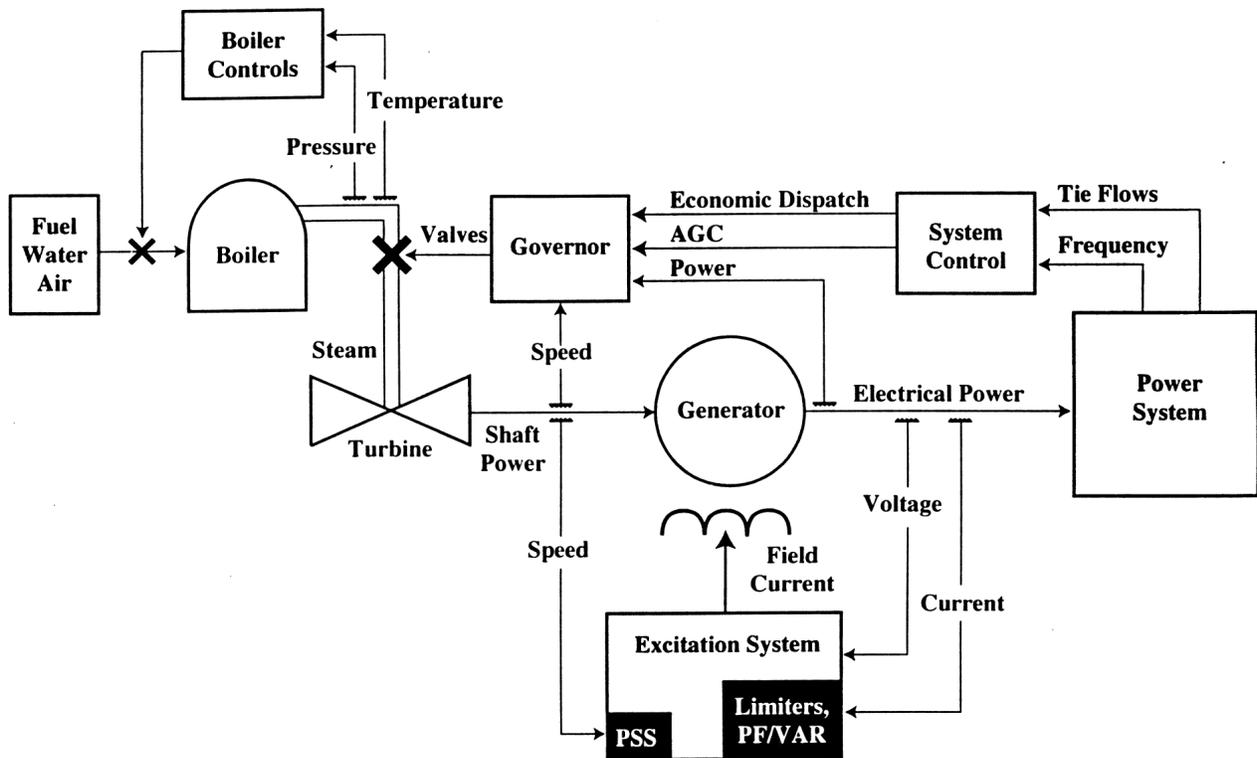
**Figure 1: Turbine-Generator Control Loops**
