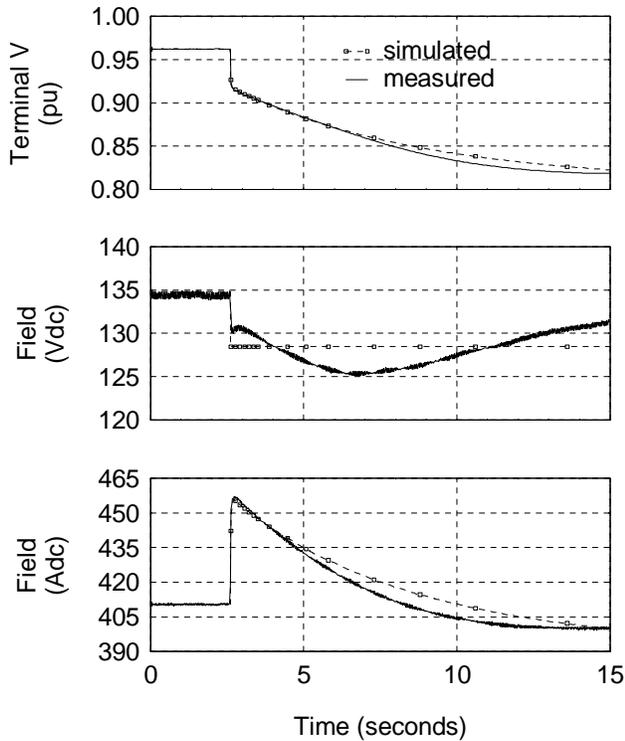
**Figure 5. 0 pf Load Rejection Test**
