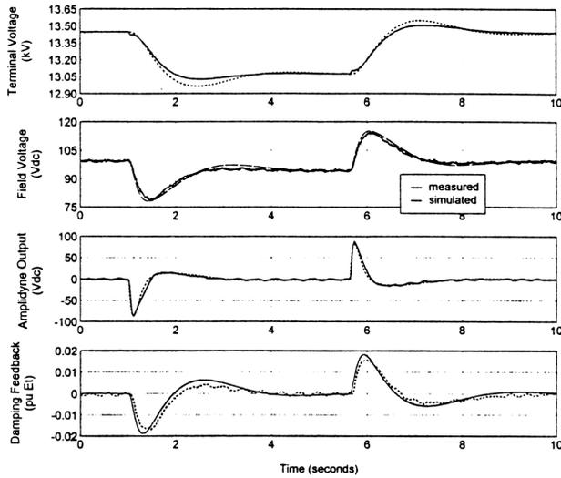
**Figure 7: Comparison of Measured and Simulated Response for Alternator-Rectifier Excitation System**
