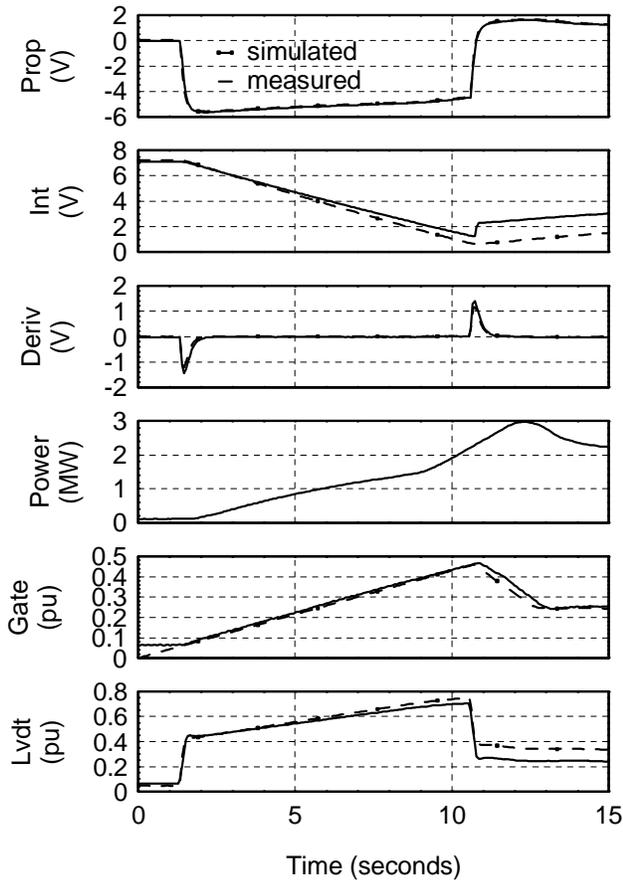
**Figure 10. PID Governor On-Line Response**
