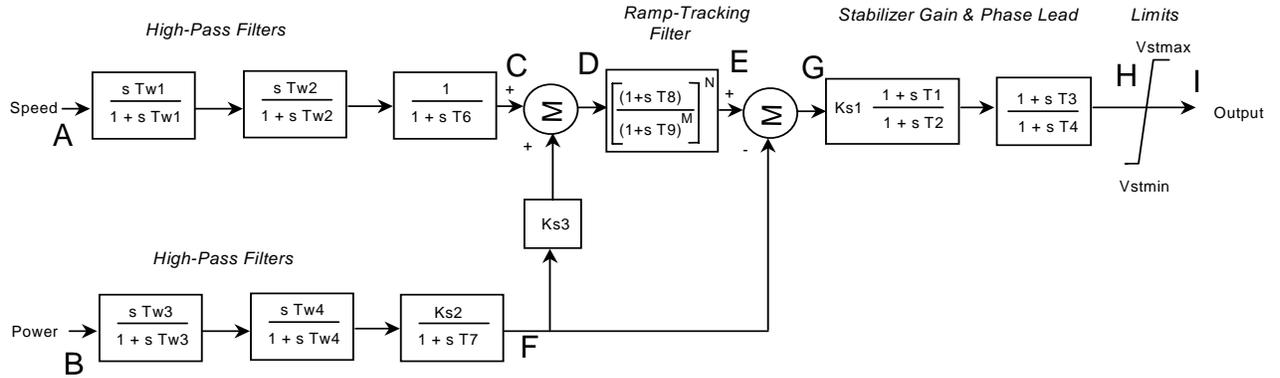
**Fig 1. Accelerating Power PSS Model (PSS2A)**
