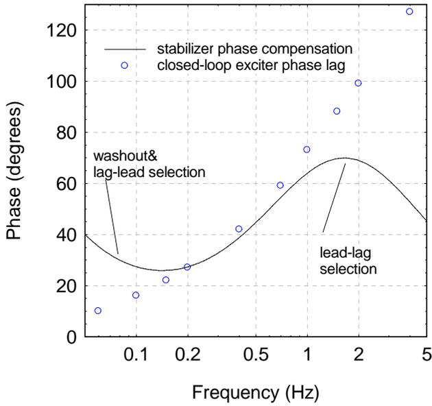
Initially, the PSS gain should be increased slowly, with transient testing at each setting. To insure sufficient stability margin, a good practice is to check the performance of the PSS with the gain increased up to twice the normal in-service setting. The objective is to ensure that the PSS gain is set at a value well below the limit at which either the exciter mode is unstable or there is excessive amplification of input signal noise.
