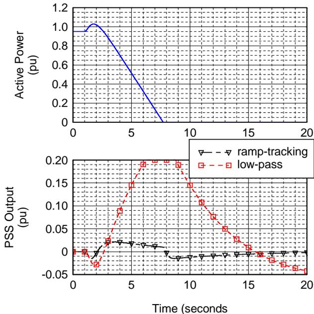
The performance of this filter may also be critical to the behaviour of the unit, in the event of inadvertent islanded operation resulting in large frequency and mechanical power variations.
