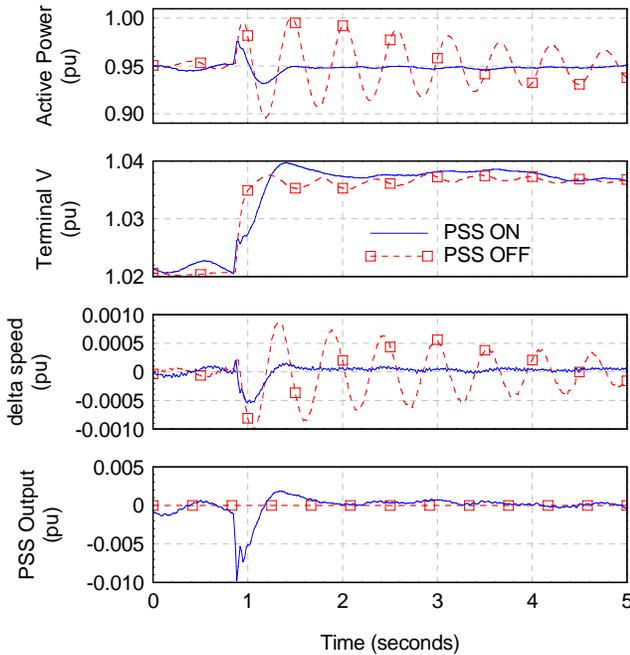
Tests and simulations performed on all types of utility-scale generators, including large and small hydro, large fossil-fired and nuclear units and combustion turbines, have consistently demonstrated that a conventional PSS tuned and tested in this manner, will improve stability for any reasonable operating scenario.
