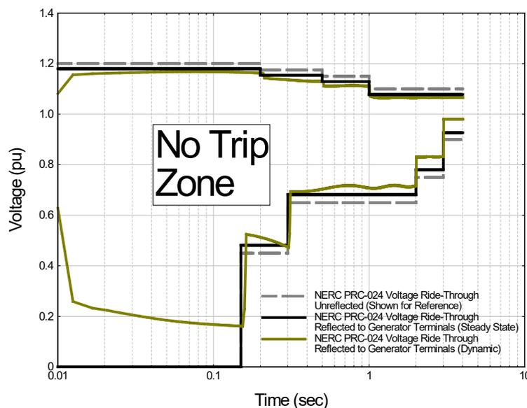
Figure 2: NERC PRC-024-3 Voltage Ride-Through Requirements for Eastern, Western, and ERCOT Interconnections, Reflected to Synchronous Generating Unit Terminals – Example
