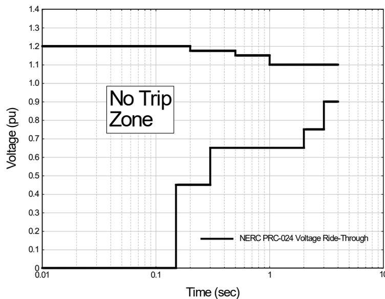
*Figure 1: NERC PRC-024-3 Voltage Ride-Through Requirements for Eastern, Western, and ERCOT Interconnections, Defined at the High-Voltage Side of the GSU / MPT*
