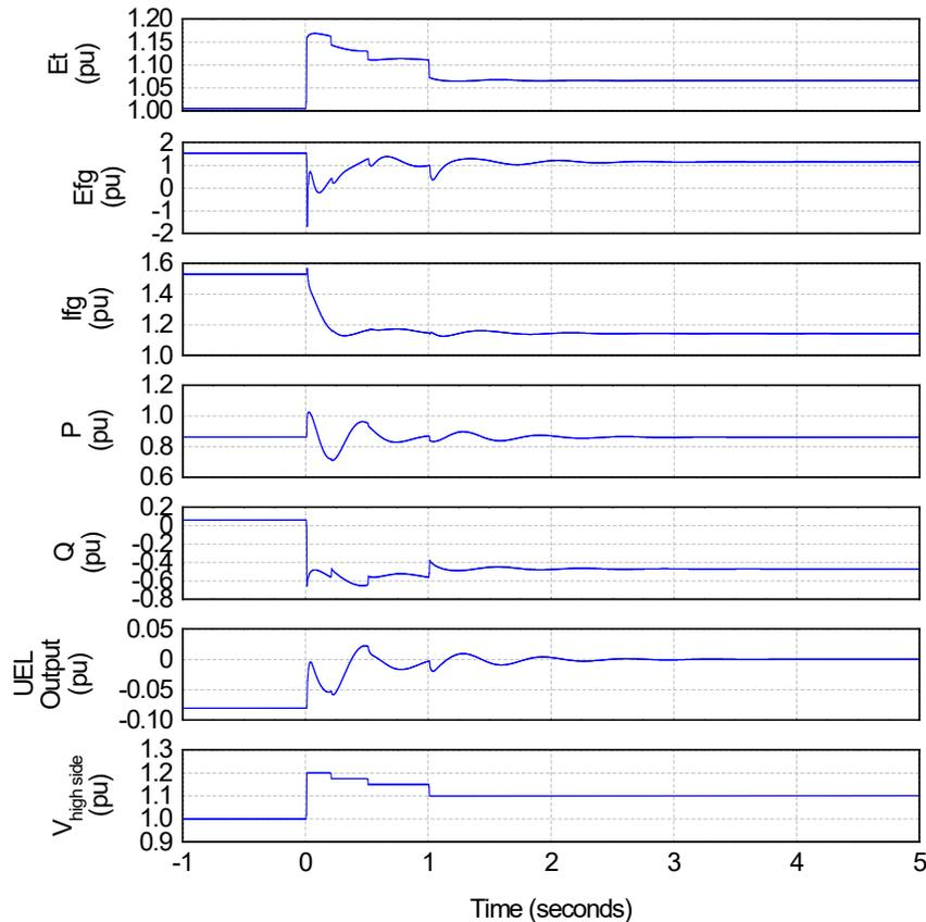
*Figure 3: Dynamic Simulation Results of the NERC PRC-024-3 High Voltage Ride-Through Requirements for Eastern, Western, and ERCOT Interconnections – Example*
