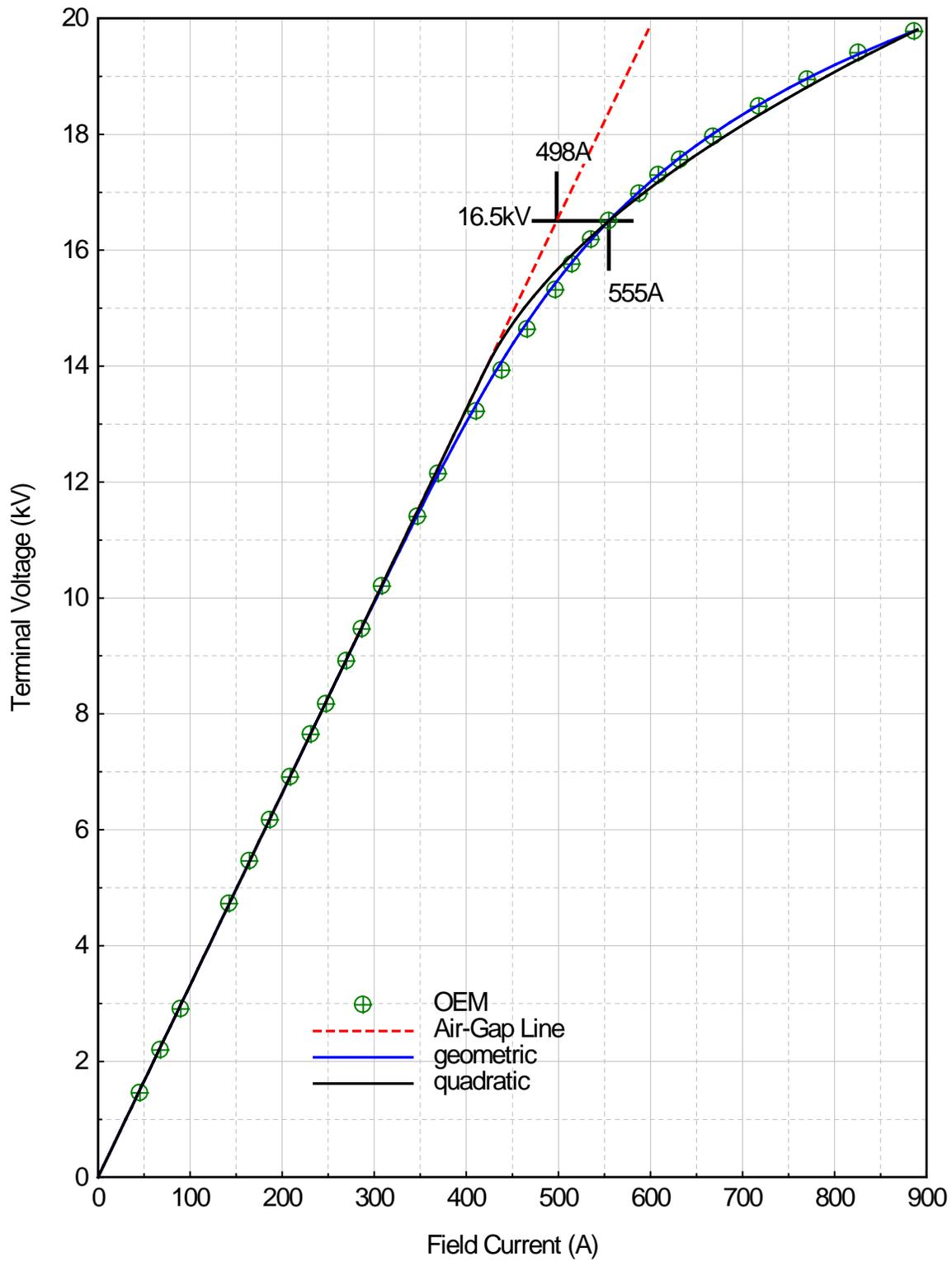
Figure 1 – Generator Open Circuit Saturation Curve
