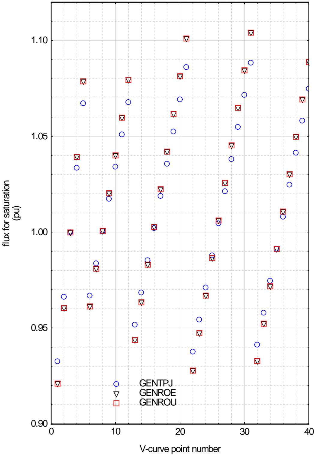
Figure 5 – Calculated Input Flux (Voltage) for the Saturation Function
