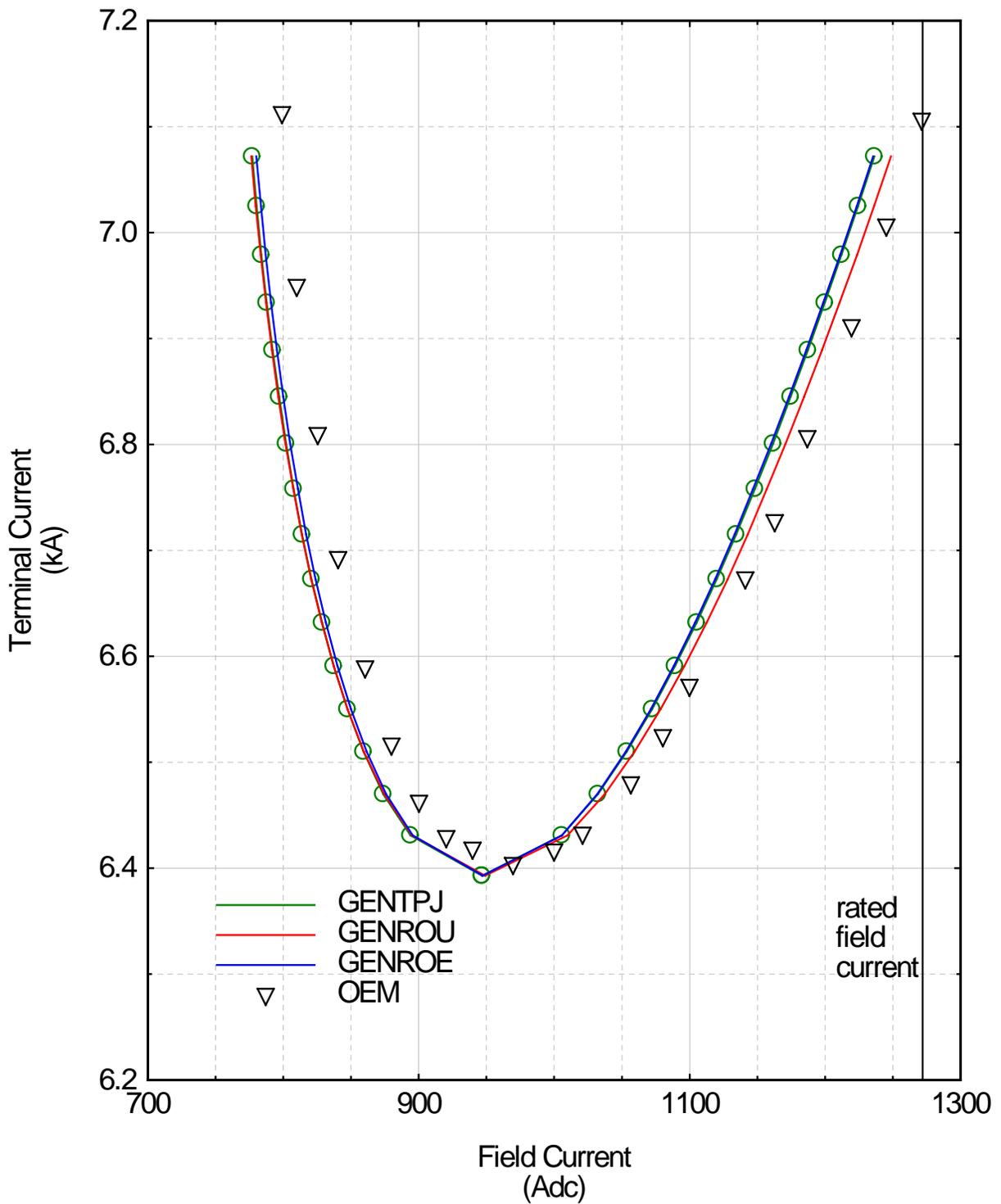
Figure 3 – Generator V-Curve for 100% (rated) Power Output and Nominal Terminal Voltage
