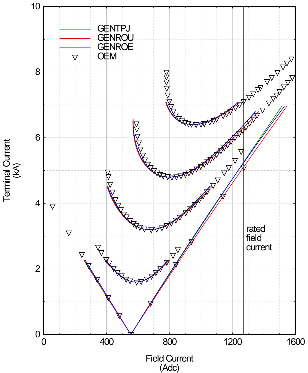
Figure 2 – Generator V-Curves for Nominal Terminal Voltage
