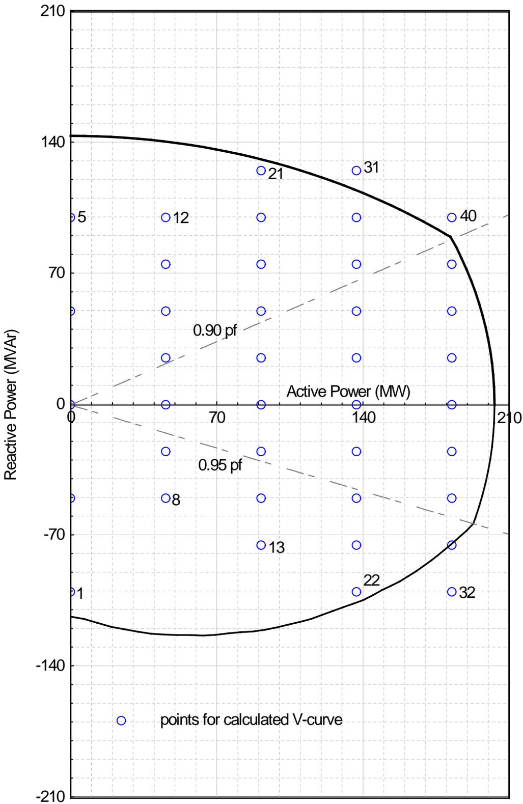
Figure 4 – Generator Capability Curve and Points Used for V-Curve Calculations
