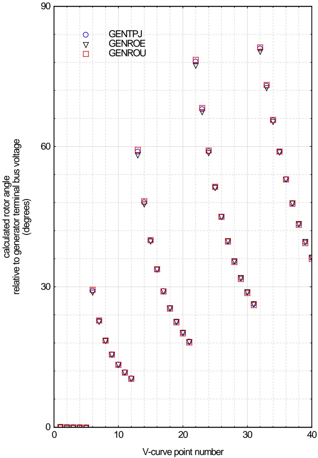
Figure 6 – Calculated Initial Rotor Angle Position Relative to Terminal Bus Voltage Angle
